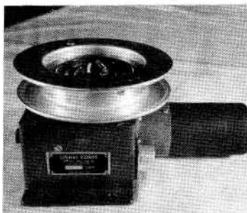
SIGNAL CORPS ANTENNA REEL
