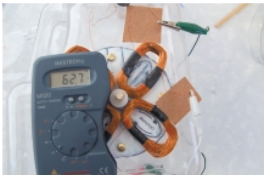
Note connection with green & white alligator clips. Note Multimeter settings readout with sound, indicating good connection.
