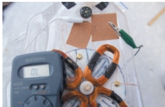
Note final Alligator Clip to the final test for connection and continuity.
