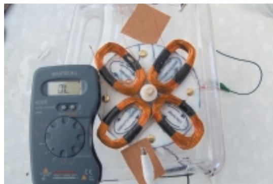
Note white alligator clip next to twisted pair. Note Multimeter readout with no sound indicating bad connection.
