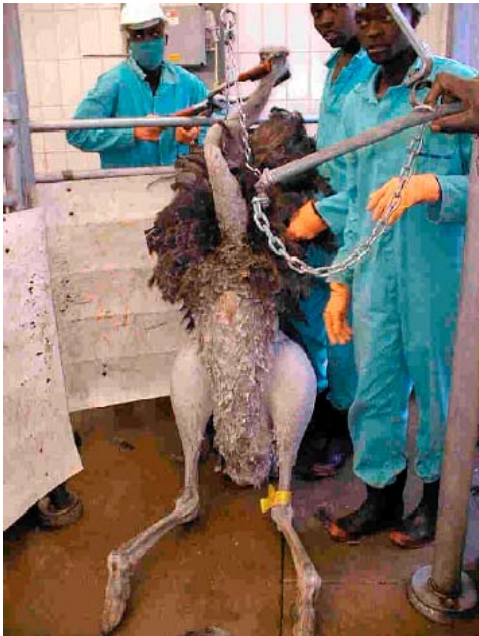
Fig. 59: Tongs for electrical stunning of ostriches
