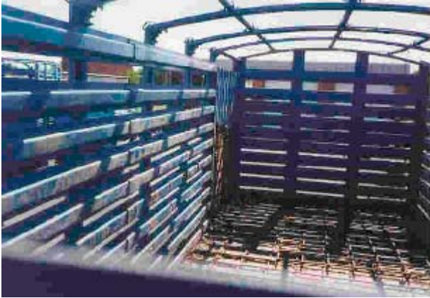
Fig. 29: Road motor vehicle for transporting cattle (cross slating of cattle truck floor to prevent slipping)
