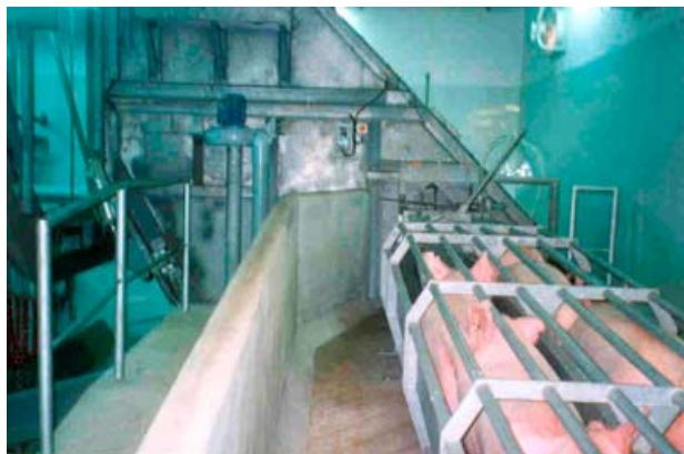
Fig. 65: Runway and entrance to a CO 2 -tunnel
