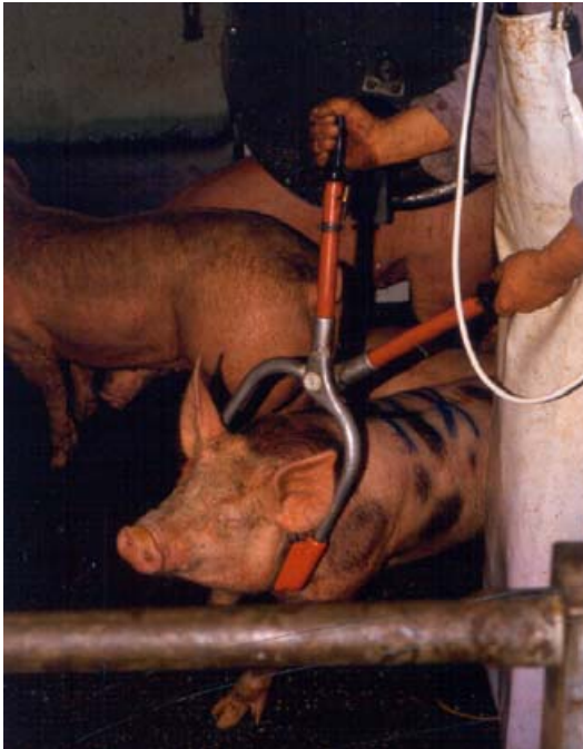
Fig. 57: Tongs for electrical stunning of pigs
