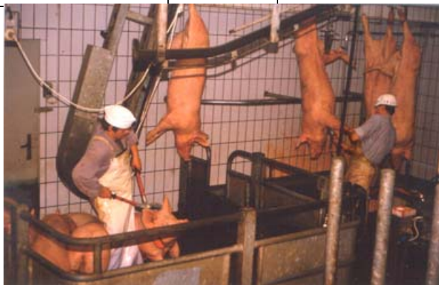
Fig. 77: Good arrangement for stunning and immediate bleeding of pigs at medium-sized
