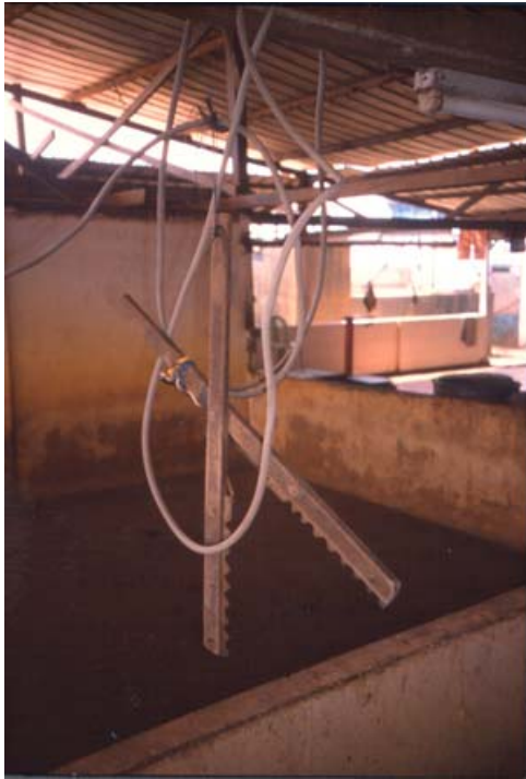
Fig. 70: Makeshift electric stunning tongs
