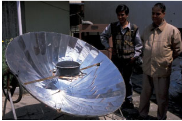
Figure 3: A solar parabolic cooker being used in Nepal ©ITDG/N. Bruce
