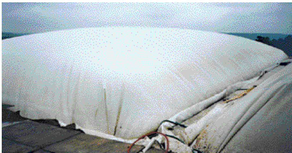
Photo 3. After two or three weeks in the digester, the odorless, dry waste can be used for cow bedding or packaged and sold as soil amendment.
