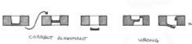
Correct and incorrect alignment of the punch
