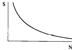
Fig. 2b. S-N no endurance limit
