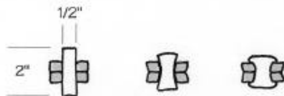
Figure 10. A cross-section of the tongs at the rivet.
