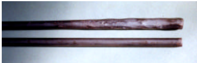
Figure 1. A comparison of 1/2" round and finished tong blank
