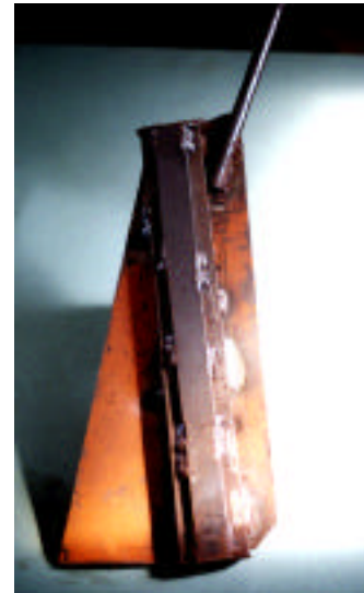
Figure 3. Original upsetting die. This die was used to make approximately 200 pairs of tongs.
