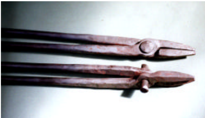
Figure 12. A finished pair of tongs, and a pair ready to be riveted.
