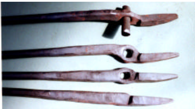
Figure 7. The forging progression—tong blank rough forged, slot punched, drifted, and rivet pin inserted.
