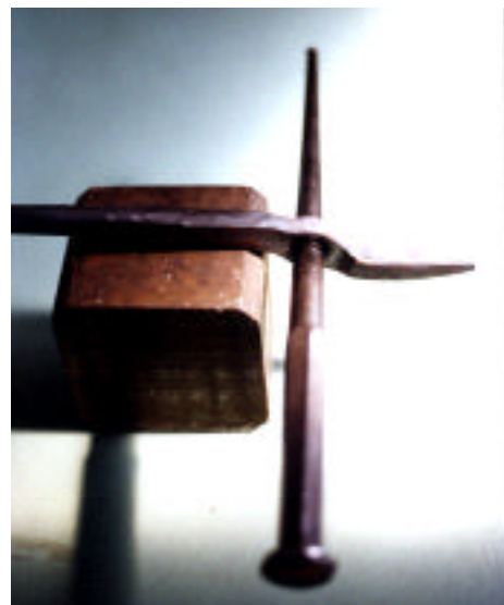
Figure 9. Showing the position of the anvil and drift while forging the third offset.
