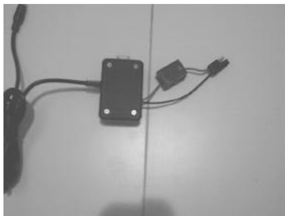
Ferrite choke on power lead:
