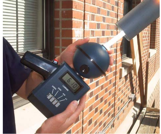
Figure 1. Spectrometer and integrating sphere
