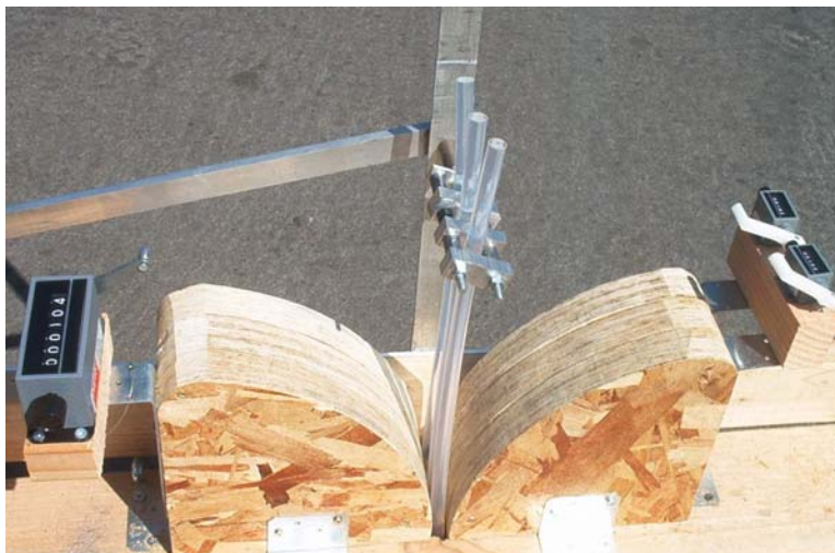
Fig. 1: Fiber fatigue testing device
