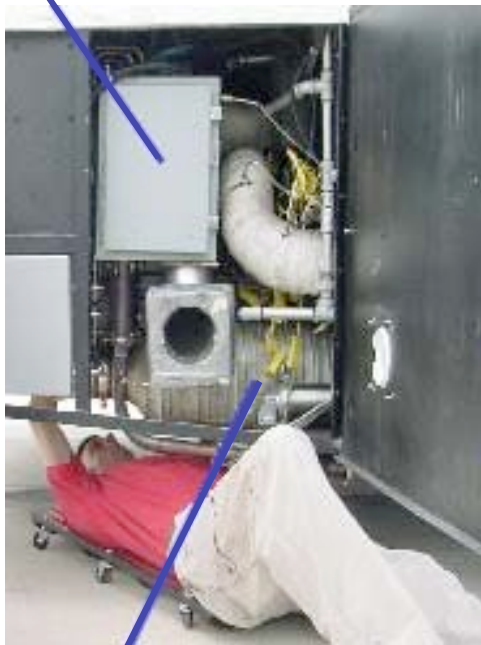
Figure 15 Picture of part of plasmatron diesel reformer system in the back of the bus
