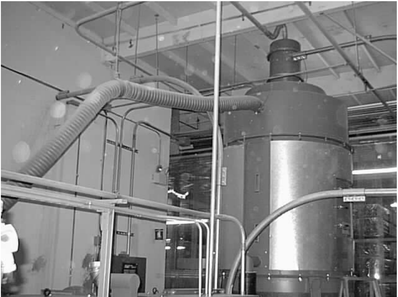
Figure 14, Material Drying Hopper
