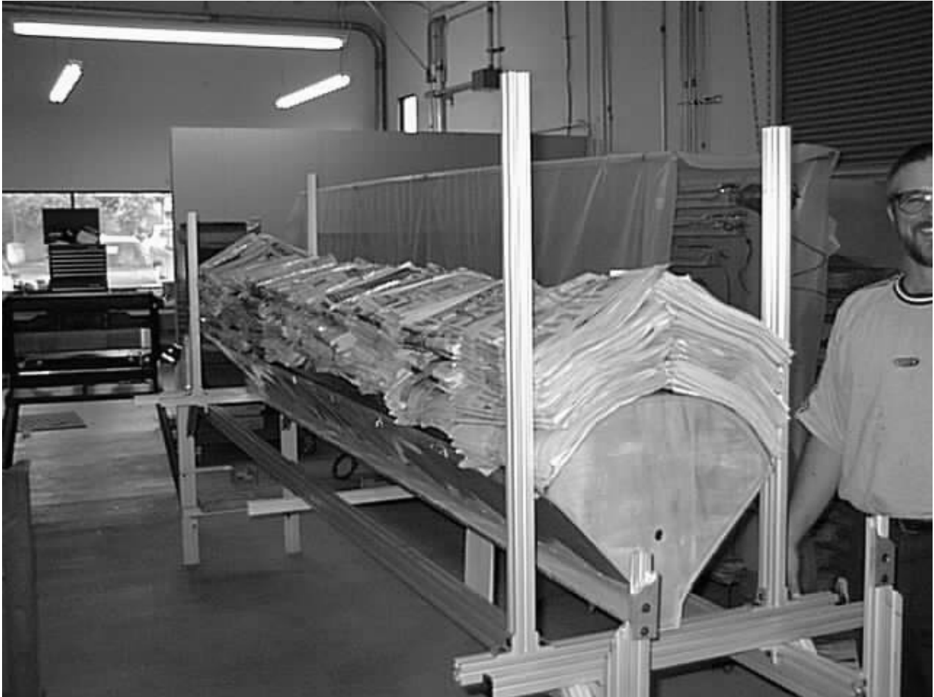
Figure 42, Prototype Module Static Test
