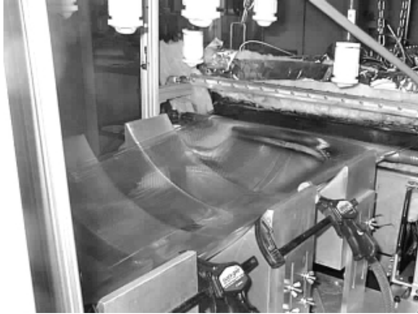
Figure 15, Lens Cold Shoes (three) With Lens Sagging Into Required Radius
