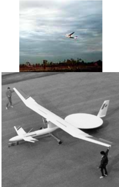
Fig. A.3.1 SHARP flight experiment and 1/8 model 10
