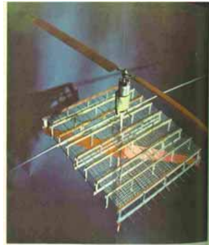
Fig. A.1.2. Microwave powered helicopter. 200 W of power was supplied to the electric motor from the rectenna that collected and rectified power from a microwave beam. 1
