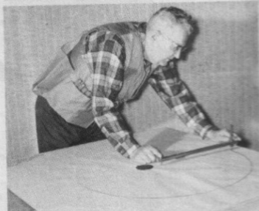
To determine pattern uniformity, also percentages, scribe a 30-in. diameter circle around the greatest concentration of pellet holes. See p. 2338 for detail
