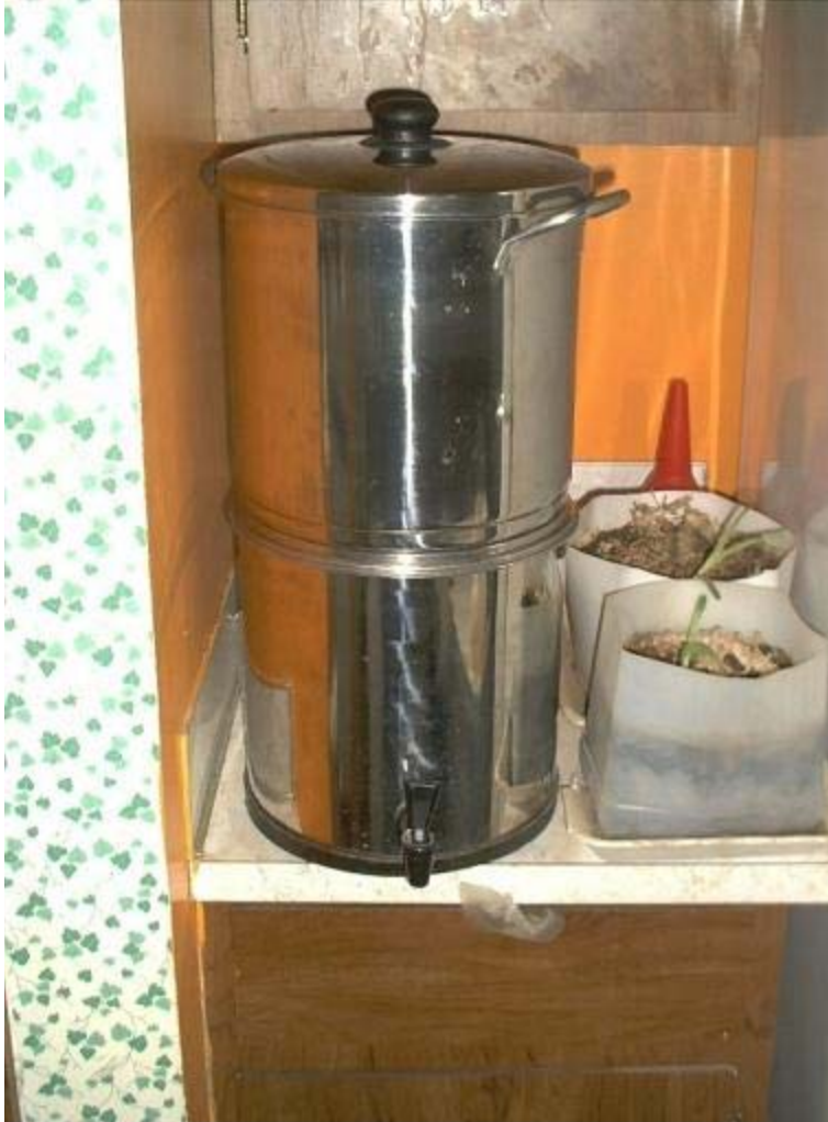
A gravity operated water filter will filter water without power or pressure.
