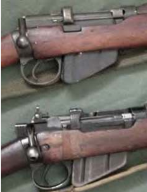
The SMLE No. 1 receiver (top) does not have the peep sight as does the No. 4 (bottom).
