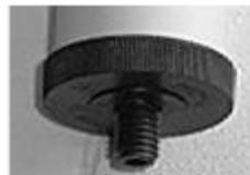
Measure this portion of the filter element. Use a drill bit of the same diameter to drill a hole in the center of the bottom portion of the coffee can.
