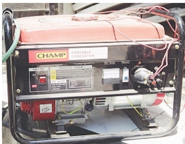
Portable generator set – a 'genset'
