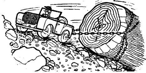
"Low ratio is used . . . on heavy ground and for heavy pulling."
