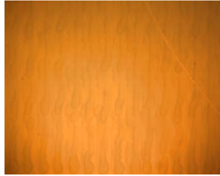
Figure 4 PEDOT on glass at room temperature.
