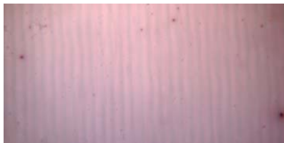
Figure 8 A portion of P3HT layer at 25°C onto PEDOT layer.
