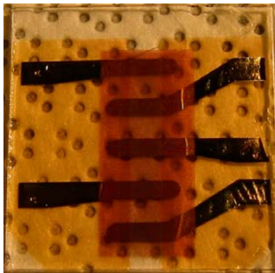
Figure 12 A completed photovoltaic device on ITO/glass.
