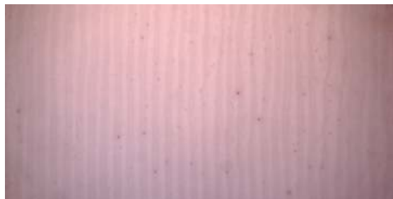
Figure 7 A portion of P3HT layer onto glass at 25°C.
