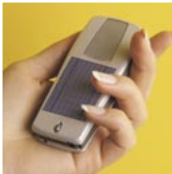
Pictured above, lightweight 0.6 Volt Sliver® cells are ideal for charging portable battery powered devices.
