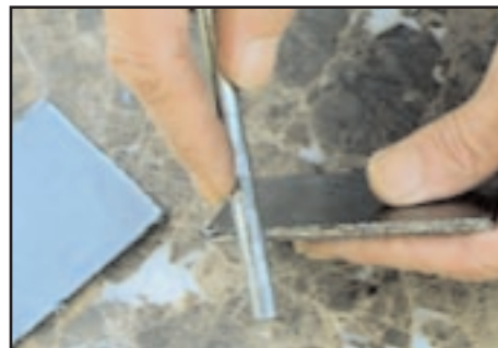
Smoothing the edges of the graphite plates with a smooth metal tool handle.
