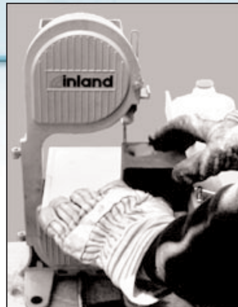
Cutting graphite blocks with wet band saw
