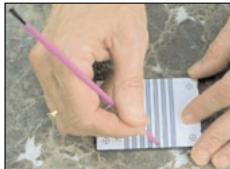
Marking the flow fields on the graphite plates
