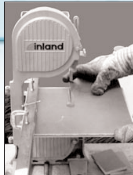
Cutting out fiberglass endplates
