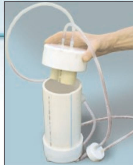
The P38 electrolyzer
