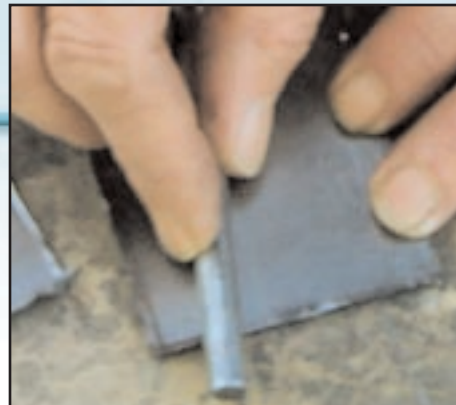
Smoothing the edges of the graphite plates with a smooth metal tool handle.
