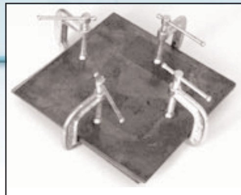
The MEA is clamped between the plates.
