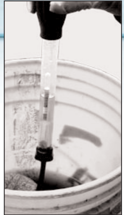
Testing the lye in the drip bucket with a hydrometer.
