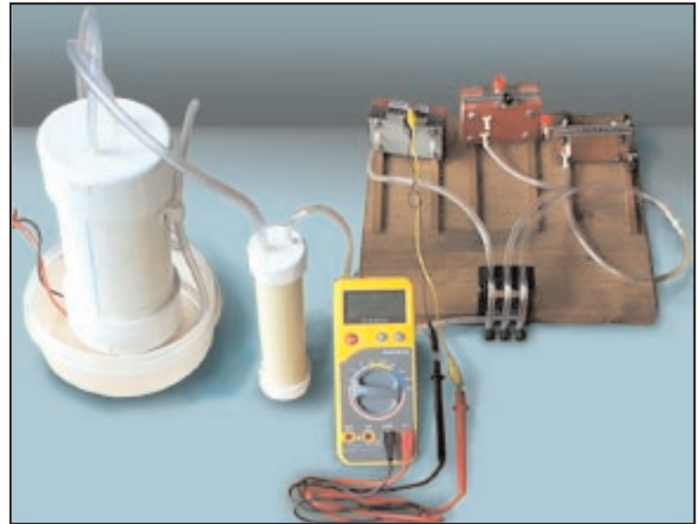
From left – electrolyzer, bubbler, meter and testing stand with 3 fuel cells.
