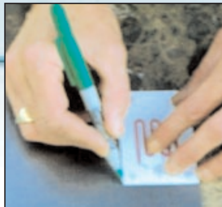
Using a template to mark the graphite foil.
