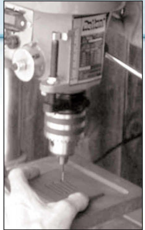
Routing the serpentine flow fields
