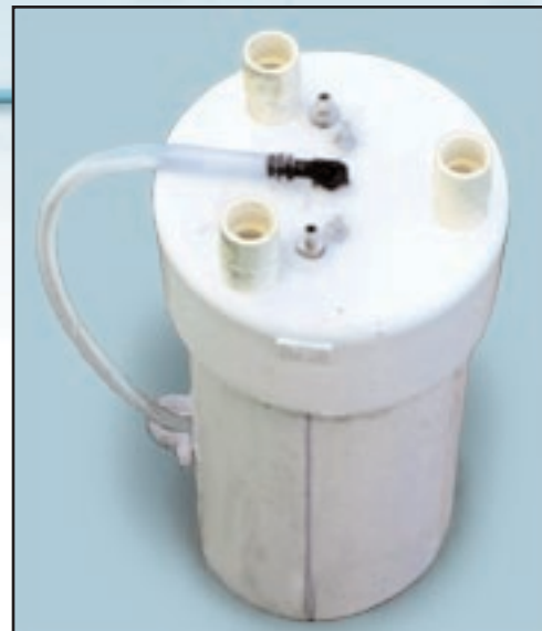
The electrolyzer upside-down, without the top cap
