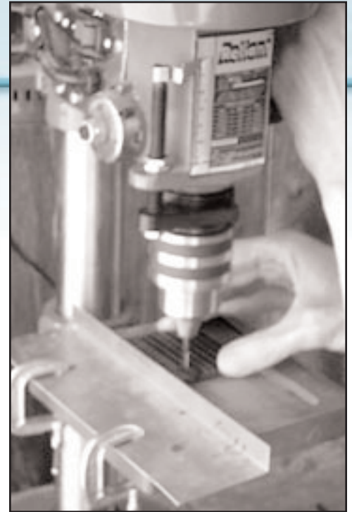
Routing the vertical flow fields
