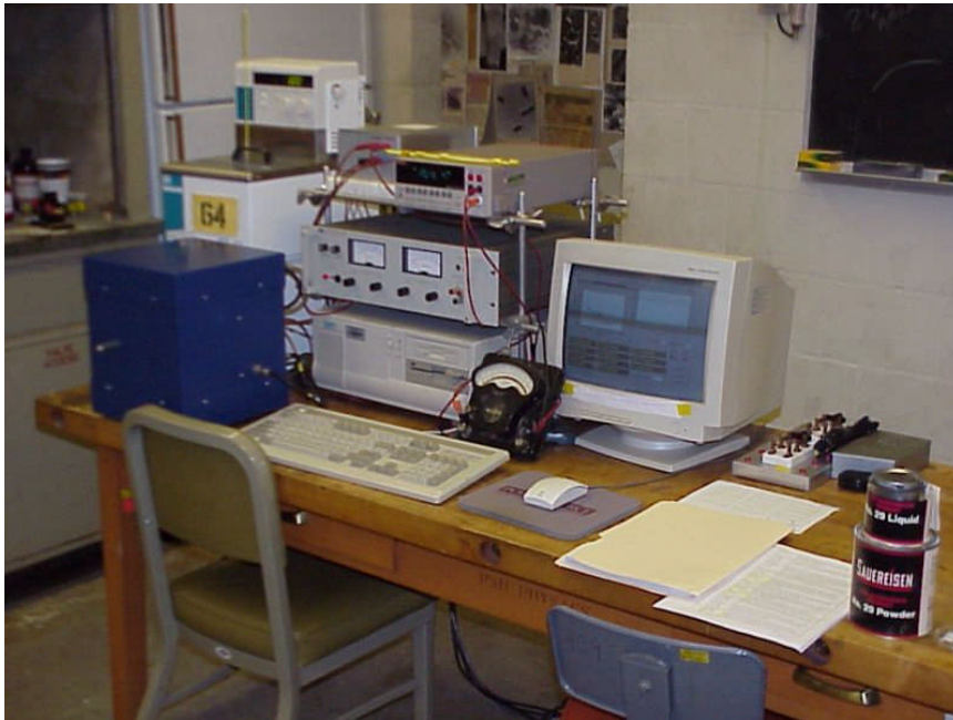
Figure 1.9. A typical cold fusion experiment, in the blue Seebeck calorimeter on the left. From J. Dash, Portland State University. Photographs by Dan Chicea, provided courtesy B. Zimmerman. This calorimeter costs $6,000. Most experiments cost roughly $50,000 including all equipment, and they are run by volunteers and retired professors. Some have produced 50 to 300 megajoules in one run. They have achieved the two goals hot fusion has failed to reach for 60 years: breakeven and full ignition.
