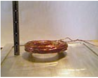
Fig. 7 Copper coil levitated approximately 10 millimeters above aluminum plate.
