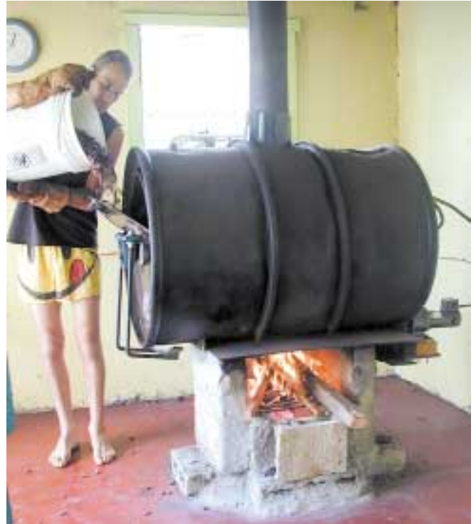
The author pouring cocoa beans into a homemade roaster. A 24 volt DC motor powers the tumbler, which allows the beans to roast uniformly.
