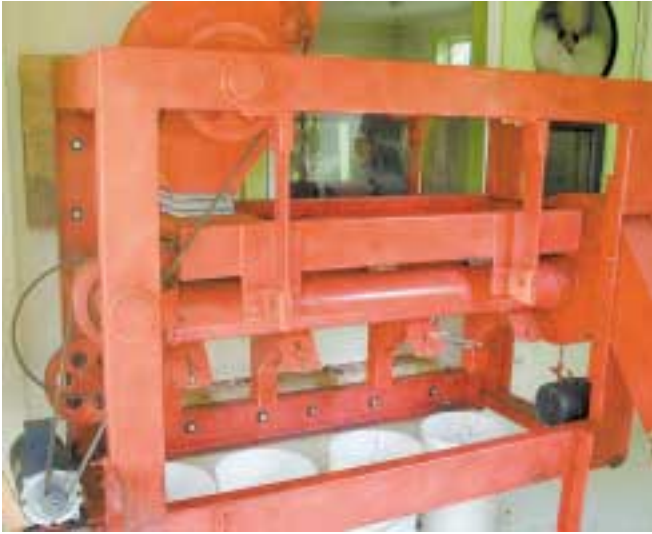
Refurbished antique winnowing machine, retrofitted with 24 volt DC motors (one motor for vibration and one motor for a powerful fan), removes the outer shell of the roasted cocoa beans.
