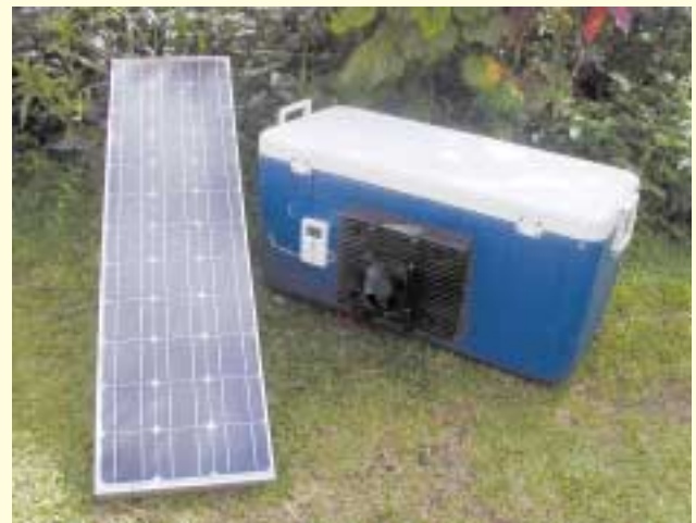
Peltier effect cooler and PV panel.
