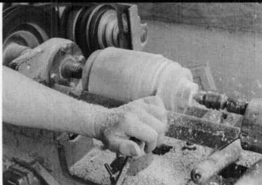
A narrow chisel forms the front bead.
