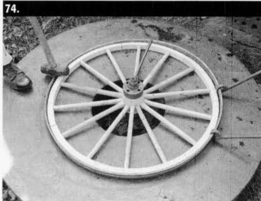
The tyre dogs are applied to the tyre and one sledge hammer holds the tyre steady and over the felloes.
