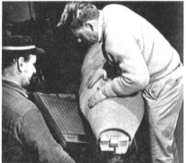
HEATER softens sheet Plyfoam for bending over the ribbands on the basic mold.
