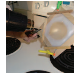
Figure G: Using a heat gun to soften the plastic stock over the frame
