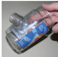
Figure D: Attaching the vacuum port (soda bottle neck)
