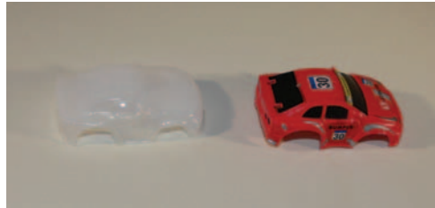
Figure A: A mini R/C car body copied with a peanut butter jar vacuum former
