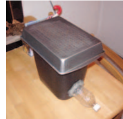
Figure M: A bigger version of the vacuum former, made from a trash can and baking pan
