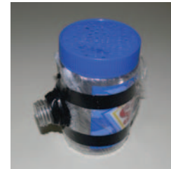
Figure F: Sealing the jar/Saran Wrap with electrical tape and attaching the lid
