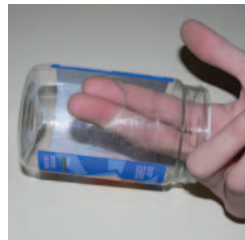
Figure C: Hole cut in side of jar to accept neck from soda bottle
