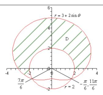
Note as well that we've acknowledged that  $-\frac{\pi}{6}$  is another representation for the angle  $\frac{11\pi}{6}$ . This is important since we need the range of  $\theta$  to actually enclose the regions as we increase from the lower limit to the upper limit. If we'd chosen to use  $\frac{11\pi}{6}$  then as we increase from  $\frac{7\pi}{6}$  to  $\frac{11\pi}{6}$  we would be tracing out the lower portion of the circle and that is not the region that we are after.
