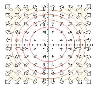
Notice that the vectors of the vector field are all perpendicular (or orthogonal) to the contours. This will always be the case when we are dealing with the contours of a function as well as its gradient vector field.
