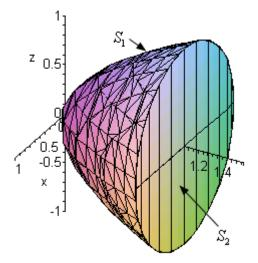
As noted in the sketch we will denote the paraboloid by  $S_1$  and the disk by  $S_2$ . Also note that in order for unit normal vectors on the paraboloid to point away from the region they will all need to point generally in the negative y direction. On the other hand, unit normal vectors on the disk will need to point in the positive y direction in order to point away from the region.
