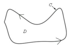
First, notice that because the curve is simple and closed there are no holes in the region D. Also notice that a direction has been put on the curve. We will use the convention here that the curve C has a **positive orientation** if it is traced out in a counter-clockwise direction. Another way to think of a positive orientation (that will cover much more general curves as well see later) is that as we traverse the path following the positive orientation the region D must always be on the left.
