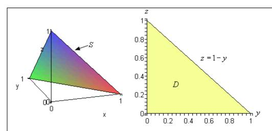
Notice that the axes are labeled differently than we are used to seeing in the sketch of D. This was to keep the sketch consistent with the sketch of the surface. We arrived at the equation of the hypotenuse by setting x equal to zero in the equation of the plane and solving for z. Here are the ranges for y and z.
