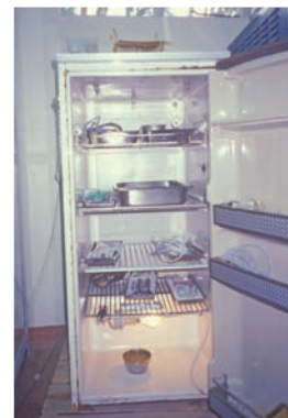
Fig 2. Formalin cabinet in well ventilated room.
