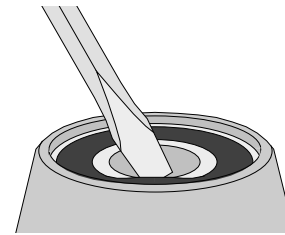
13.9 Removing the seal from the bearing.
