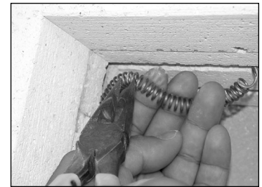
If the element is too long, squeeze the coils together slightly.
