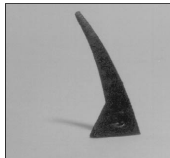
An under-fired cone.
