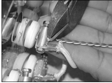
Tighten the element connectors according to step #14. Then cut off the element ends.
