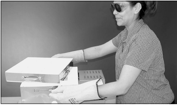
To look at the glass during firing, move the top slightly. Look inside the kiln for a second or two. Wear firing safety glasses and gloves.
