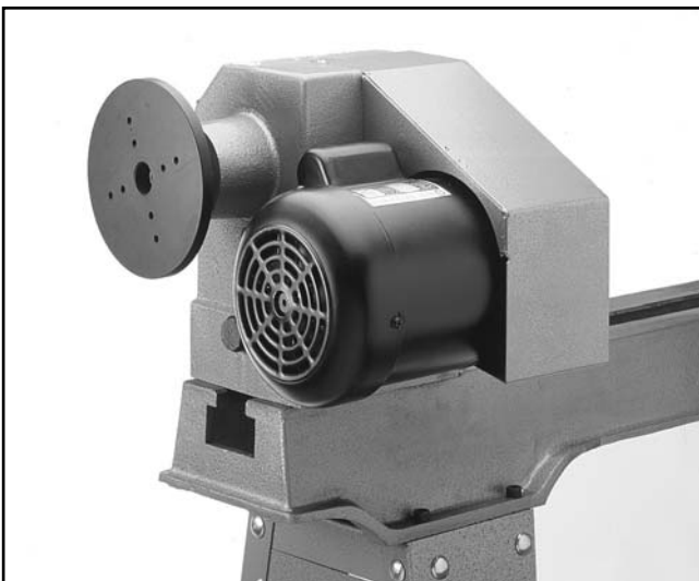
Figure 17. Headstock set at 180°.
