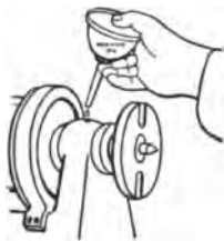
FIG. 76. — OILING SPINDLE OF A MACHINE.
