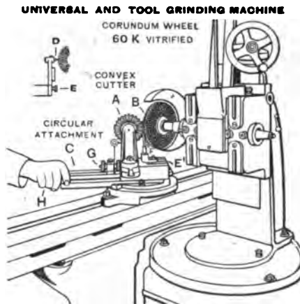
FIG. 33. — GRINDING CONVEX CUTTER.
