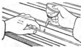
FIG. 77. — OILING WAYS OF A MACHINE.
