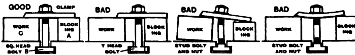
FIG. 31. — METHODS OF CLAMPING WORK. GOOD AND BAD. DIFFERENT KINDS OF PLANER BOLTS.
