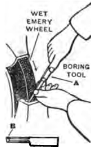
FIG. 67. — GRINDING BORING TOOL.
