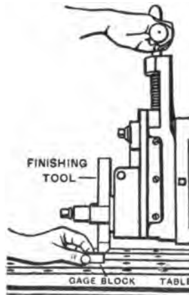
FIG. 25. — GAGE BLOCK TO SET PLANER TOOL.
