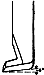
FIG. 4.— LEFT DIAMOND-POINT PLANER TOOL.
