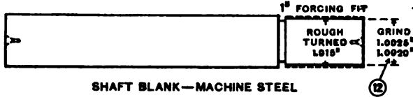
SHAFT BLANK—MACHINE STEEL FIG. 14. — SCHEDULE DRAWING.
