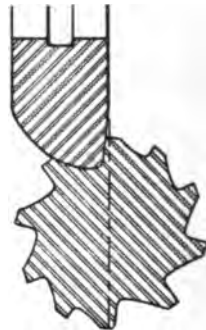
FIG. 49. — FORM OF FLUTE IN REAMER FOR BRASS. TEETH WITH NEGATIVE RAKE, IRREGULARLY SPACED.
