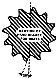
FIG. 19.—TEETH OF HAND REAMER WITH NEGATIVE RAKE.
