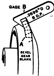
FIG. 12. — MARKING DEPTH ON BEVEL-GEAR BLANK.
