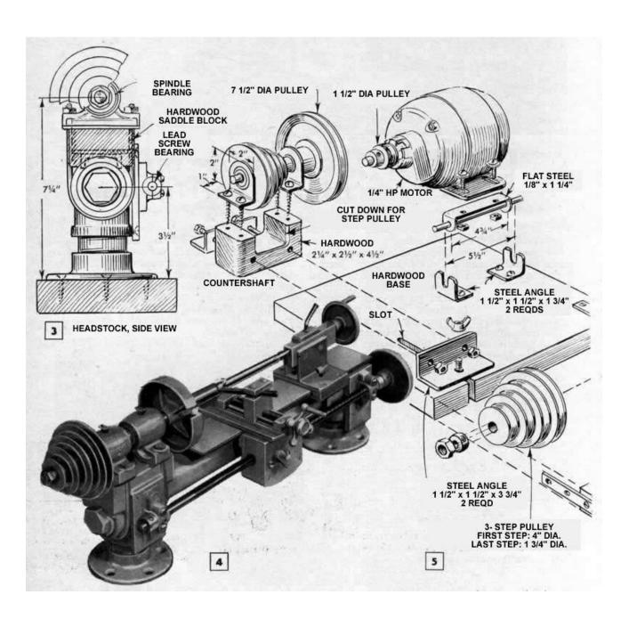
The headstock-spindle bearing (Figure 5) are held on the pipe tee by means of U-bolts and a saddle block of hardwood. One face of the saddle is shaped to the contour of the tee; the other is faced with a 1/8" steel plate on which the pads of the pillow blocks rest. The purpose of the steel plate is to make it easier to align the bearing sleeves when the assembly is bolted in place. Cut the saddle about 1/8" thicker (about 21/2") than indicated. Then assemble the parts temporarily.
