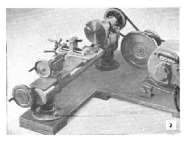
Screw the parts tightly together and then mount on a hardwood base as in Figure 5. Later, when the countershaft, motor and motor mount are added to the assembly, a second piece is attached to the first, making an L-shaped base as pictured in Figs. 1 and 2.
