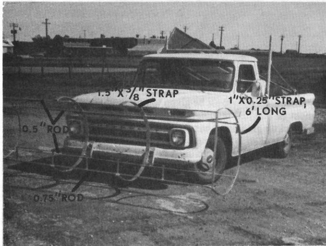
Fig. 1. A pickup grass seed stripper frame ready to cover.
