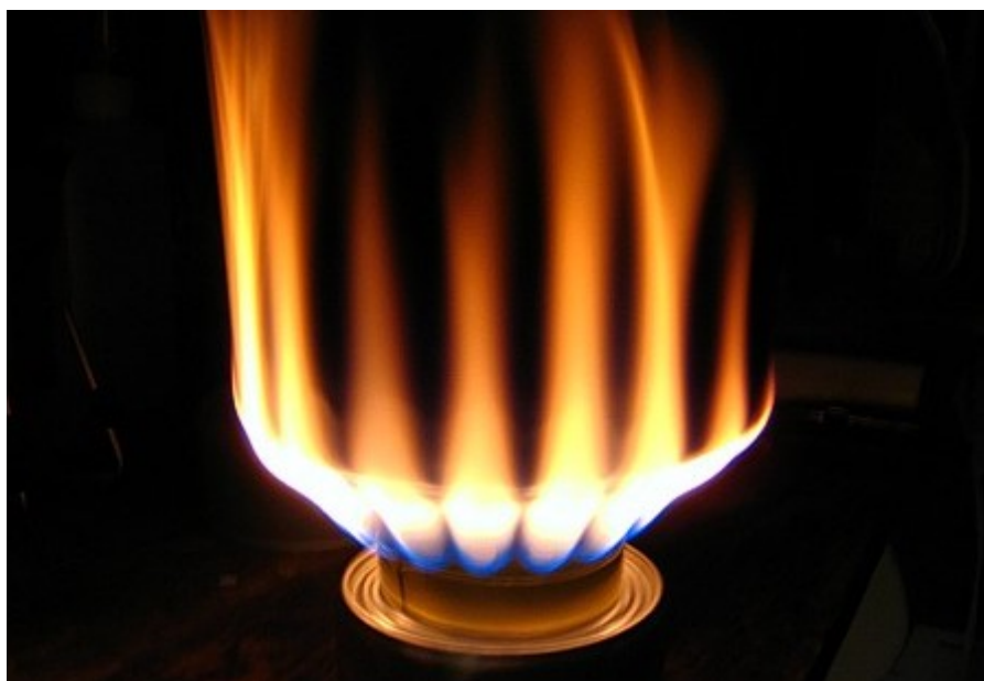
Red Iso-Heet burns with a yellow, sooty, low-temperature flame (+)
