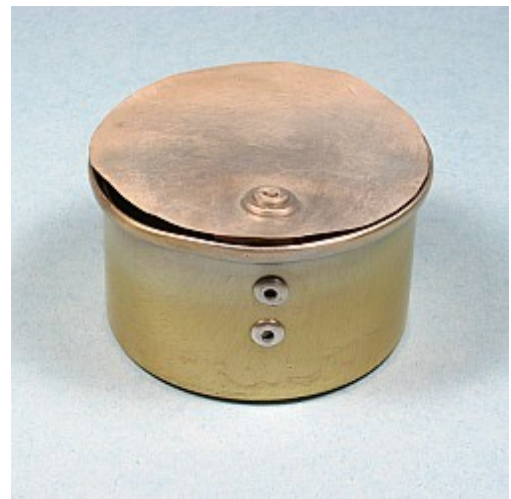
Fully-closed position (+) (Note the "L" bracket rivets on rear wall)
