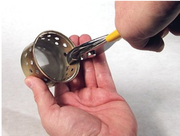
Flattening vent hole collars (+)
