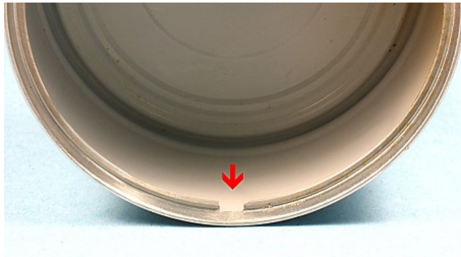
A small notch filed into the inside rim of a snuffer cup can assist with fuel recovery (+)
