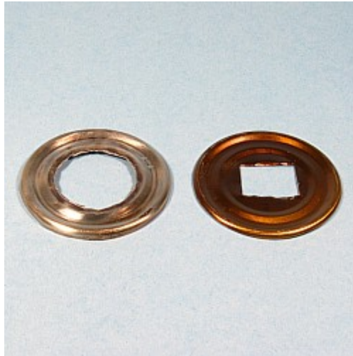
These priming caps were made from the bottoms of 3 ounce pet food cans (+)
