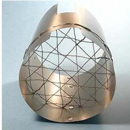
Burn platform created by stringing 22 gauge steel picture hanging wire among tiny holes punched 1" apart (+)
