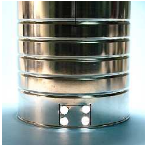
3/8" holes drilled near the corners of the ventilation port (+)
