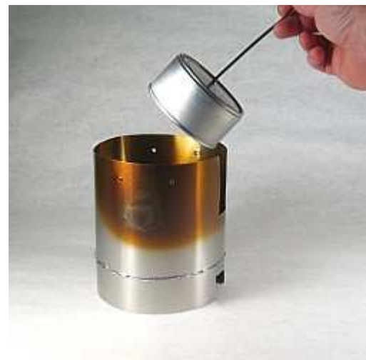
Lower the cup at an angle to direct flames away from your hand (+)
