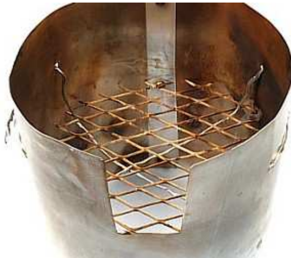
Optional grate positioned on top of sling to improve stability (+)
