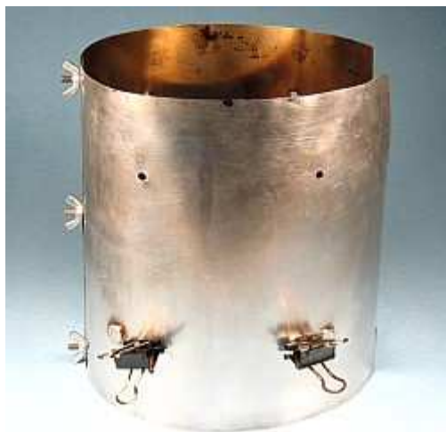
Small binder clips secure support rods (+)
