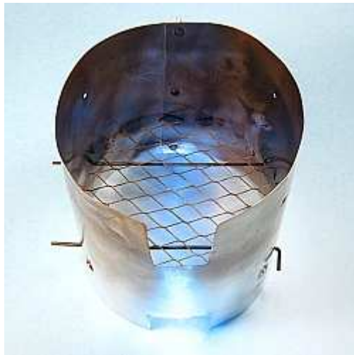
Top view shows burn platform (+)
