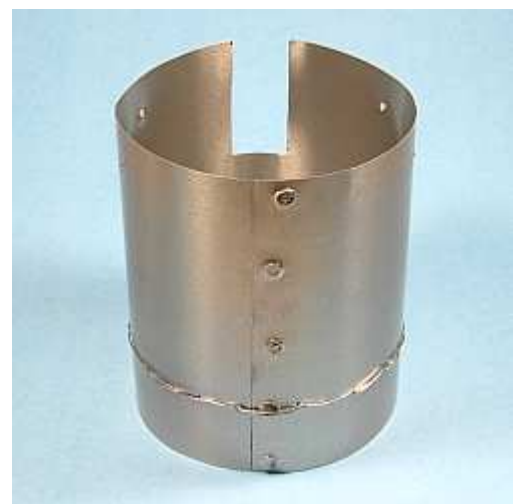
Permanently assembled model fastened with pop rivets (+)
