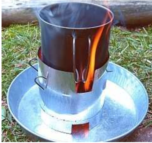
During this test burn, flames from a wood fire exit the top opening directly onto the pot handles (+)
