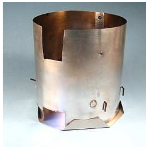
Floor in place under Fire Bucket (+)
