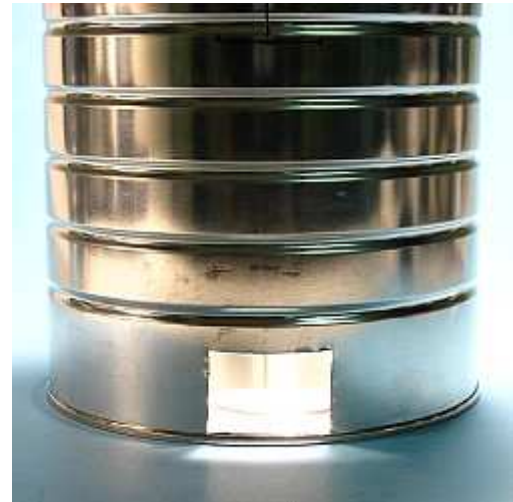
Opening cut from hole-to-hole using a jigsaw equipped with a metal cutting blade (+)
