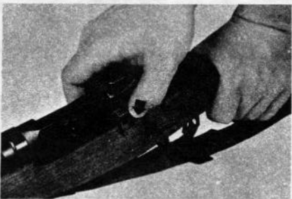
Figure 5. Locking the bolt to the rear.
