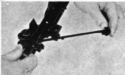
Figure 17. Replacing the connector assembly.
