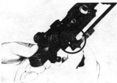
Figure 13. Removing operating rod.
