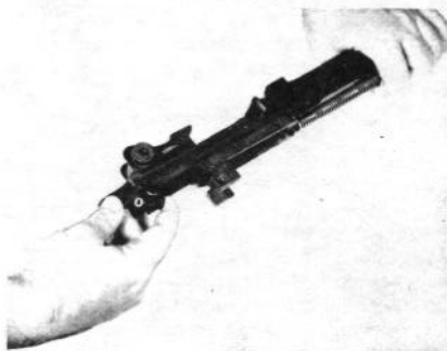
Figure 11. Removing the connector assembly.
