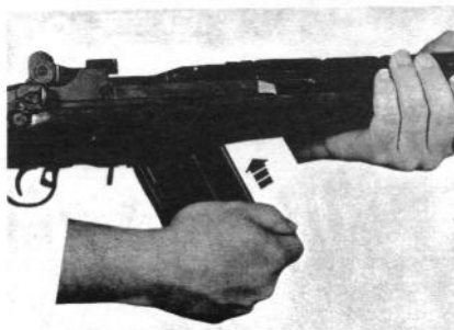
Figure 29. Loading the magazine into the rifle.
