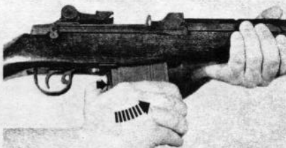
Figure 4. Removing the magazine.
