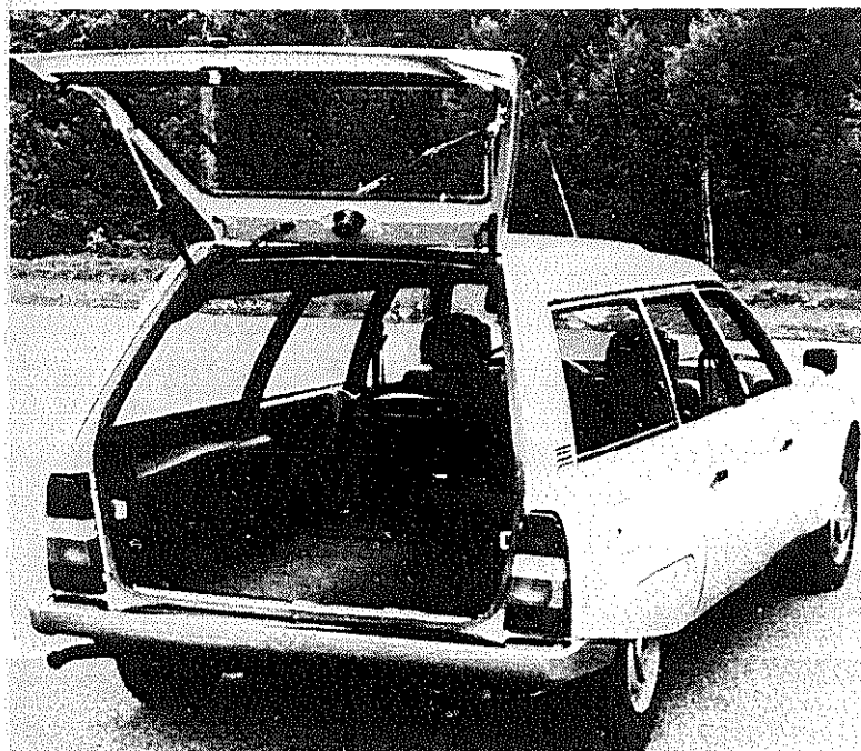
One of the largest station wagons available anywhere, the Citroen CX Diesel can carry 3/4 ton and gets 35 miles per gallon. The CX is the first high production safety car, and has the lowest air resistance of any. Despite slick appearance, it has bad-road abilities nearly as good as 4-wheel drive machines. Americans are not allowed to import them.
