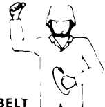
LOCK THE CRAWLER BELT ON SIDE INDICATED BY RAISED FIST - TRAVEL OPPOSITE CRAWLER BELT IN DIRECTION INDICATED BY REVOLVING FIST LEFT TURN
