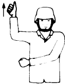
RAISE THE BOOM AND HOLD THE LOAD
