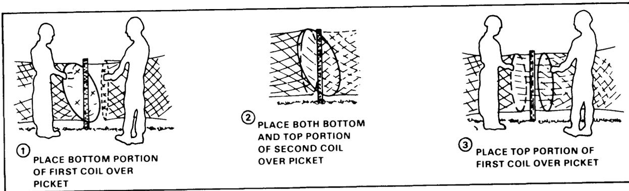
Figure 3-8. Joining concentina
