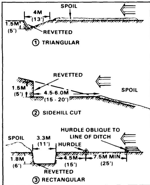
Figure 3-15. Antitank ditches
