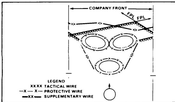
Figure 3-3. Schematic layout of barbed wire entanglements in a defensive area
