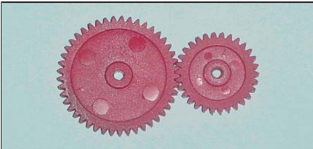
FIGURE 1.2 Properly mated gears have the same gear pitch (modulus)
