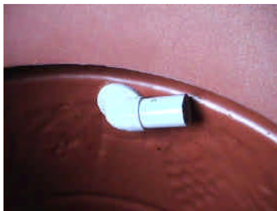
I experimented with angling the pipe of the overflows to determine the water-level inside the filter. Later, after final assembly, I took them all out again, applied a generous helping of Fernox jointing compound to the inside and outside faces, and the flexible hoses before re-fitting.
