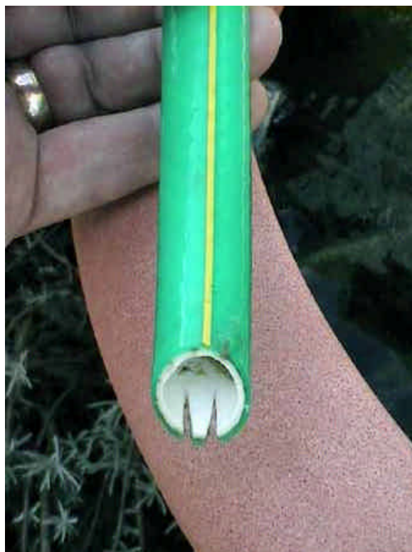
Close-up of the Zik type of toothed venturi. This really swirls and chops the air into the water as it passes, and makes quite a loud noise.
