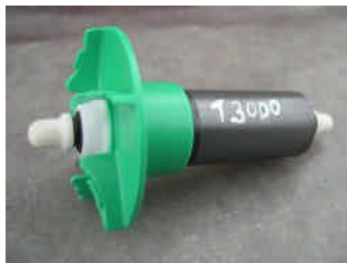
The Titan 2000 and 3000 impeller is the same, but without the cap. Note the little lugs on the
