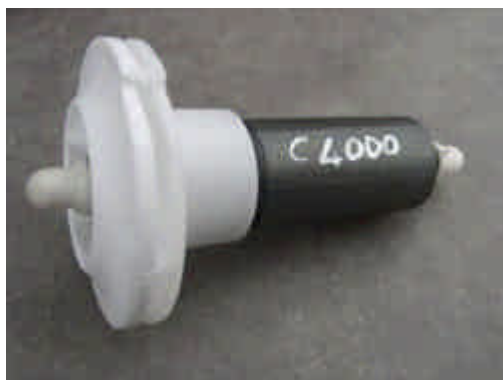
The Cascade 4000 impeller has a cap over the impellers vanes. Water is drawn in from the front (left-
