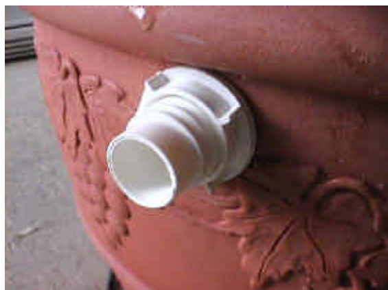
Drill to accommodate the 22mm pipe fittings for the one inlet and the two overflows. Notice how I had to fit it between the raised decorative pattern to ensure a flush fit.
