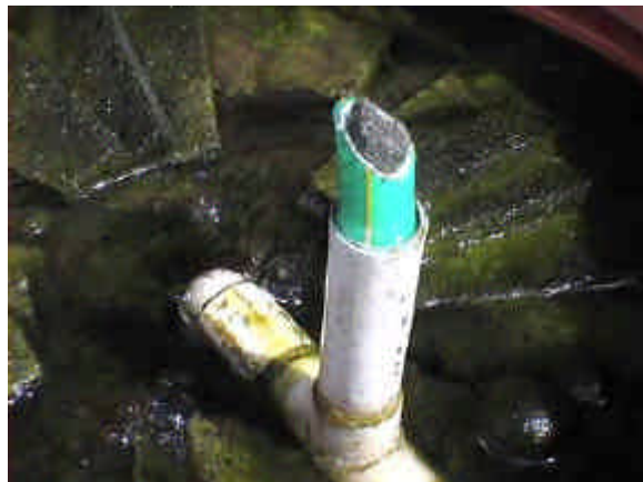
Close-up of the Zik-type venturi, with a piece of green-scrubby acting as an air and noise filter.
