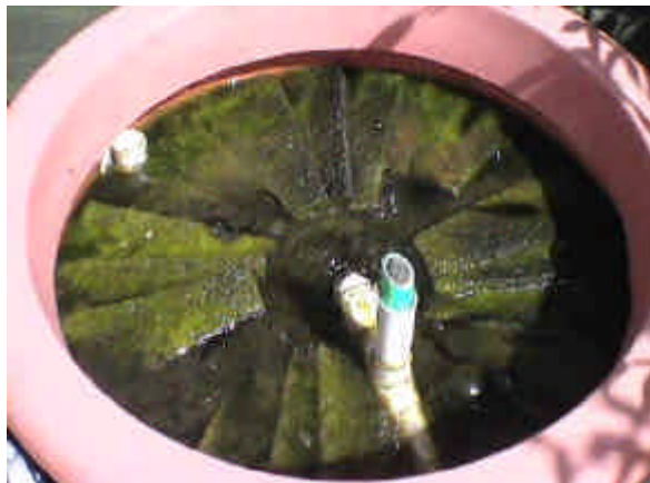
The new-cut scrouper pad filters in the bio-filter with the Zik design of venturi aerating the water.
