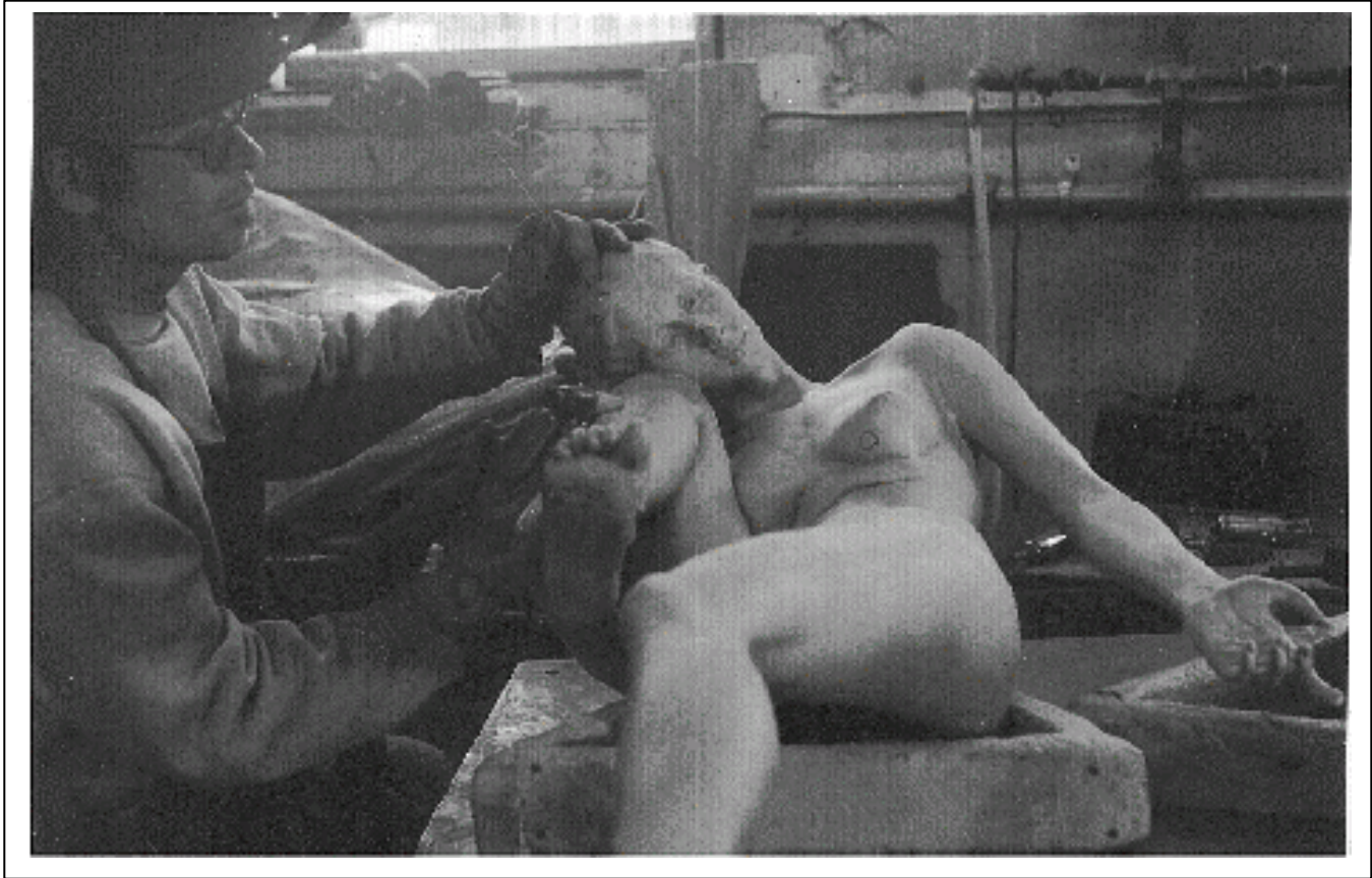
Picture 3. Here the work begins. It is know as de-vesting the casting, sandblasting, cutting sprueing off the sculpture with a body grinder, reciprocating saw, or plasma cutter. You will inspect the metal for flaws in the metal, which have to be repaired, and do a lot of precise welding. I'm using a heli arc or TIG welder to join the pieces of a full body lifecasting.
