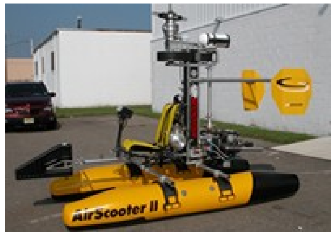
Ultralight helicopters can also be outfitted with pontoons, for amphibious use.
