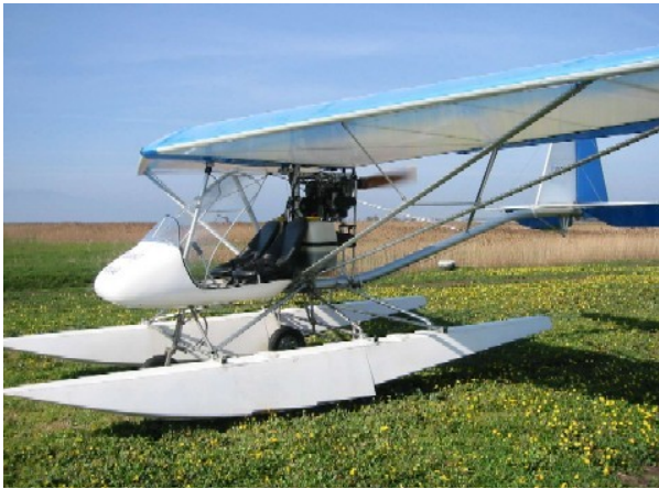
Float Planes: Many ultralights can be turned into little float planes, with the addition of optional pontoons.
