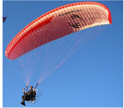
Paramotor: This is a parasail parachute, with a motorized harness, and optional landing gear.
