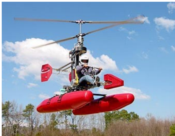
Ultralight helicopters can also be outfitted with pontoons, for amphibious use.
