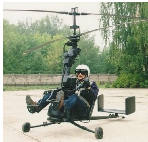
The smallest helicopter designs are now not much larger than the pilot.
