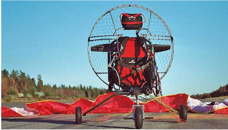
Paramotor: This is a parasail parachute, with a motorized harness, and optional landing gear.
