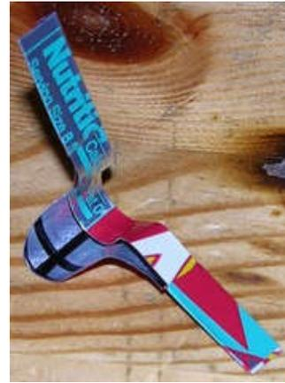
Padlock shims are one way to open a padlock without the key (they are used in pairs), and they can also be improvised from empty soda cans, or beer cans, like the example on the right.
