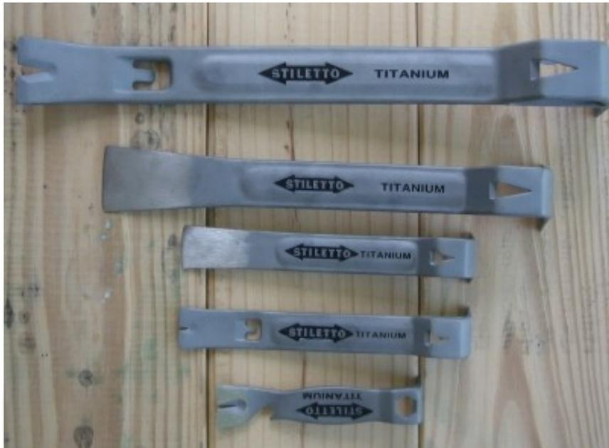
Titanium is stronger than steel, non-magnetic, and never rusts.
