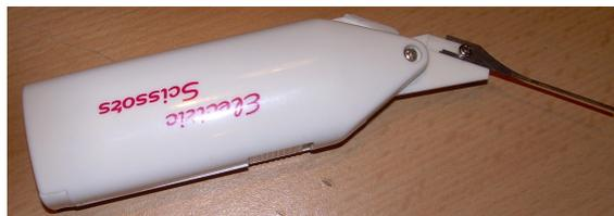
Here is a pen-style pick gun, and an improvised one, made from electric scissors.
