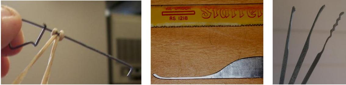
Here is a wire snap pick, with a rubber band spring, and picks made from hacksaw blades.
