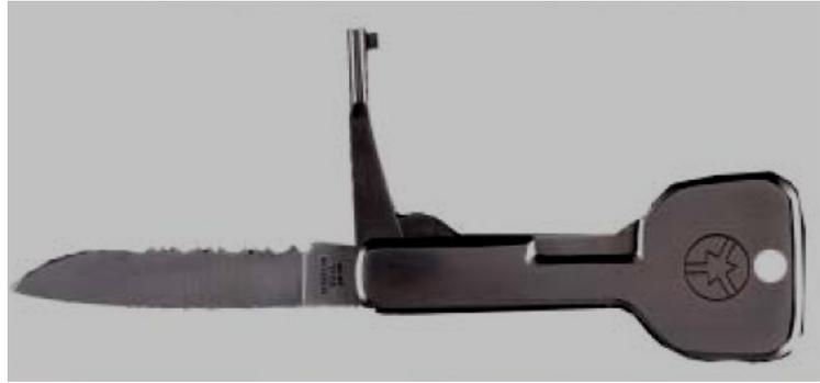
Shown here are a key with a tiny knife blade, and another with a blade and a handcuff key.
