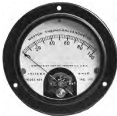
PLATE XVII. Thermo Galvanometer for use with Decremeter. Weston Electrical Instrument Co.
