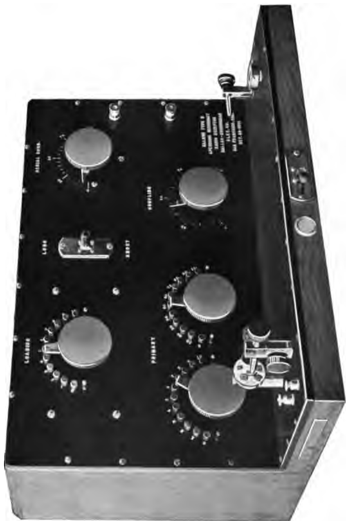
PLATE XXVIII. Short Wave Untuned Secondary Receiver. (Crystal Detectors.).
