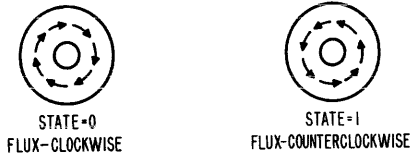
Fig. 5-1. Magnetic cores are used as memory stores.
